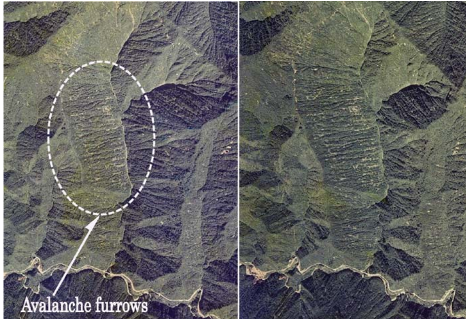
Fig. 4 Avalanche furrows in the Uonuma area; aerial photograph, taken during a snow-free period (September 1976, by the Geographical Survey Institute). Possible use stereo vision with 3D.
