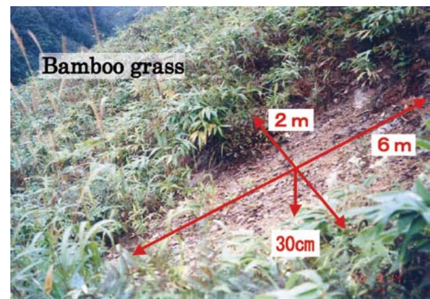
Fig. 15 Ground surface of avalanche patch in Toikanbetsu area (September 2000, by Imanishi N., Hokkaido university).
