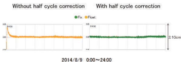
Fig. 10 GPS and BeiDou kinematic solutions of zero baseline at Etchujima, Tokyo on August 9, 2014, between JAVAD DELTA and Trimble NetR9 receivers.
